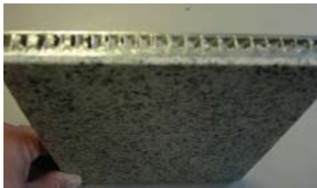
Figure 10.6 – Example of honeycombed metal backed stone fused to the stone. This stone type can only be installed with an epoxy adhesive.
