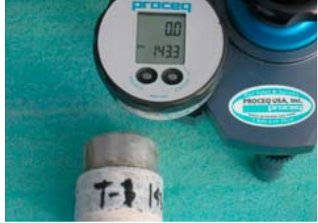
Figure 12.8 – View of cored stone and adhesive section. In this instance, failure occurred at the waterproofing membrane to substrate interface at approximately ~143 psi (1 MPa) (very good results).
