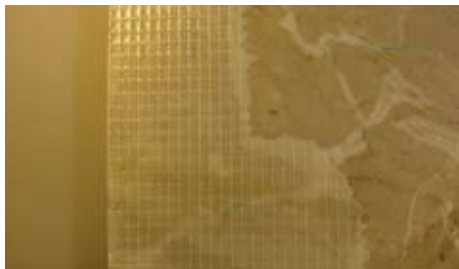
Figure 10.5 – Example of resin backed stone. Polyester resin mesh backing applied to the stone. Notice how easily the backing has peeled away from the stone itself.
