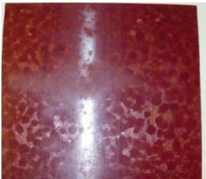
Figure 10.4 – Example of resin backed stone. Integrated polyester resin backing fused to the stone.
