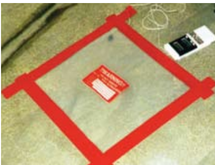
Figure 4.22 – ASTM D4263 – Plastic Sheet Method – 18" x 18" (45cm x 45cm) sheet of plastic is tightly taped to the substrate and allowed to sit undisturbed for 24 hours. If water or condensation is observed, then a measure of moisture vapor transmissions is present. This test will not provide a quantitative moisture vapor emission rate.
