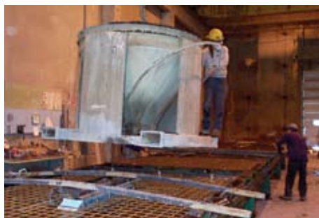
Figure 7.9 – Negative Cast Method. Concrete is poured and vibrated over the panels. A slurry bond coat consisting of LATICRETE® 211 Powder mixed with LATICRETE 3701 Mortar Admix can be used as a bonding agent between the tile backs and the concrete pour.
